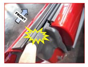
The noise occurs when the door glass is moved/rolled up and/or down with the door closed.
